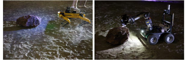
Figure 4. Spot and Husky performing tasks in the ESA ESRIC Space Resources Challenge. Spot explores the challenge area and finds potentially interesting rocks to be analyzed (left), while Husky later on independently analyzes these rocks (right).
